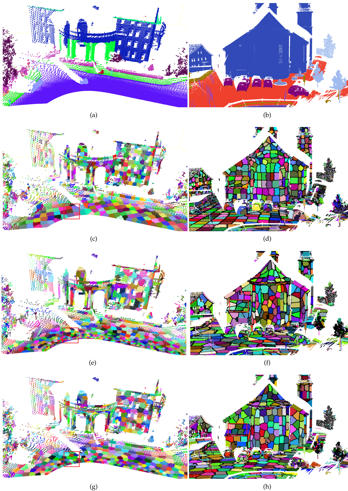
Figure 14. Visual comparisons using the point clouds from the Oakland (left) and Semantic3D (right) datasets. (a,b) Ground truth; (c,d) the VCCS results; (e,f) the BPSS results; and (g,h): our merge-swap results. Unlabelled points are not shown in the ground truth.
